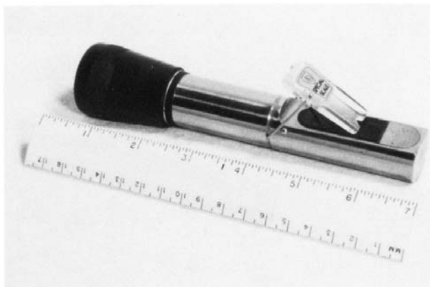
FIG. 1 Typical Hand-Held Refractometer
